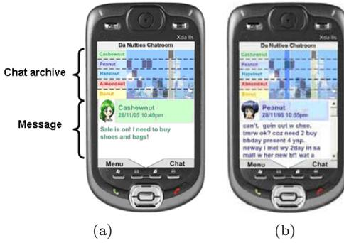
Figure 1: 1(a) Externalisation with 5 chatters and non-scrollable turn, 1(b) Externalisation with 5 chatters and scrollable turn
